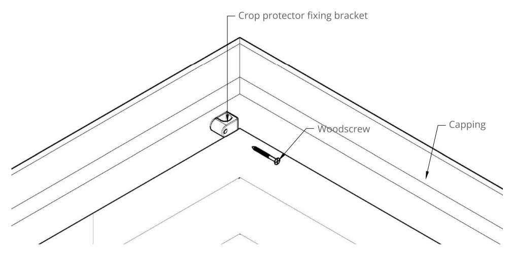
Crop protectors are to be placed in every corner of the raised bed **attached to the capping** and **above** each buttress for raised beds over 2250 mm
